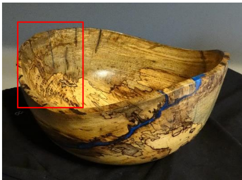
Photo 1: Hackberry bowl and expanded view to highlight blue stain and the compartmentalization in the wood. (Note that the bright blue line in the bowl is epoxy filling a large void.)
