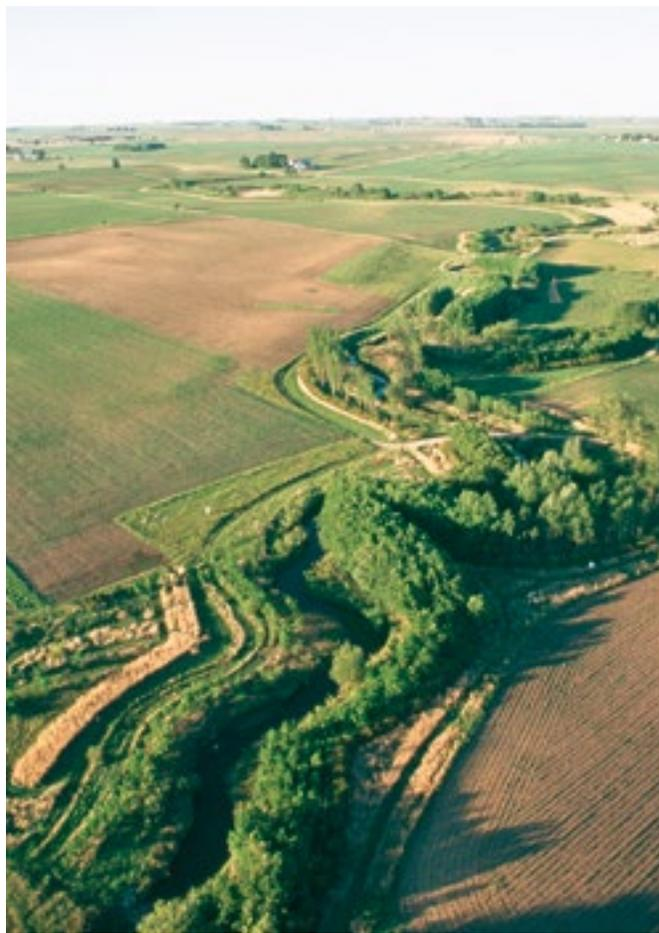
**Figure 8.6** - Multiple rows of trees and shrubs, as well as a native grass strip, combine in a riparian buffer to protect this riparian area.. Image courtesy of NRCS.
