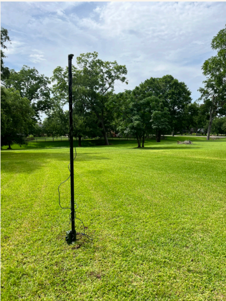
Acoustic monitor mounted on PVC pole Photo by Monica Taylor
