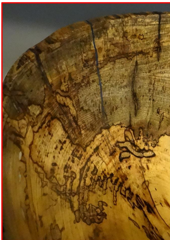
Photo 1: Hackberry bowl and expanded view to highlight blue stain and compartmentalization. Note that bright blue in the bowl is epoxy filling a large void, though blue stained wood is natural.
