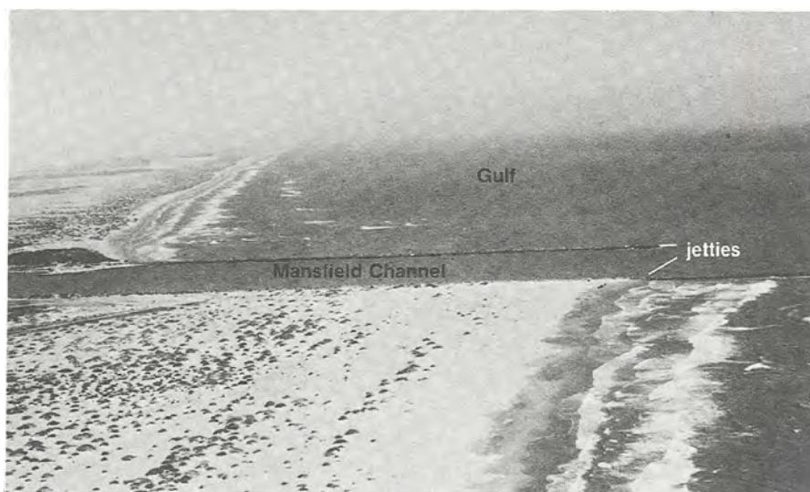
Figure 24. Jetties at Mansfield Channel. View is toward northwest. Note that sediments have accumulated on the south side of the jetties, which indicates that net longshore drift is northward at this location. Erosion has occurred on the north, or downcurrent, side of the jetties. The jetties are located in grid C-21 on plate 1.
