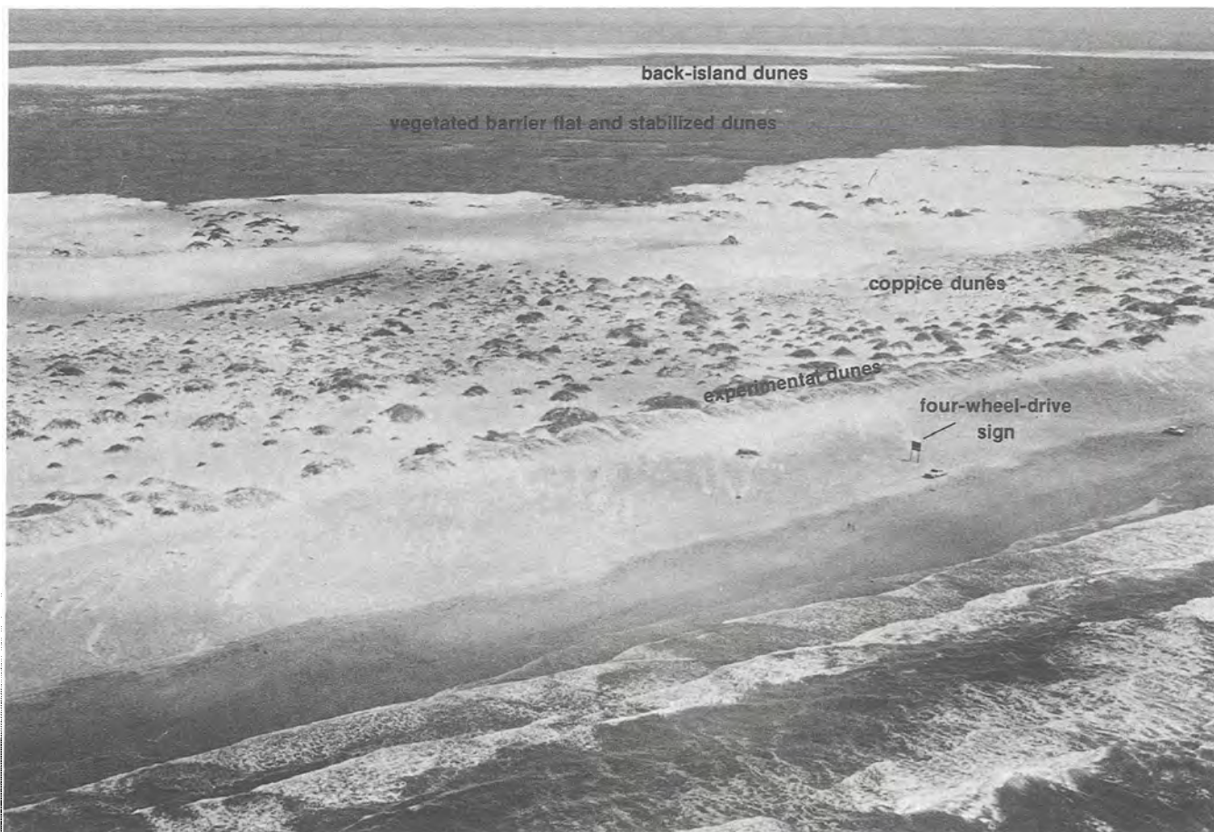
Figure 67. Experimental fore-island dune ridge. View is toward the northwest. The dune ridge that lies parallel to and along the back edge of this beach was formed by vegetation that was planted to trap and accumulate the sand blown from the beach by onshore winds. This particular dune ridge, one of a series that was artificially established, is located in the area of the four-wheel-drive sign, which is visible in the photograph (see pl. I, grid K-4, for location of sign). Note the streaks of dry, white sand that have formed downwind from clumps of vegetation on the backbeach. These accumulations of sand show effects of the onshore winds that were blowing when the photograph was taken. Also note that sand piles up along the dune ridge, but where there are gaps in the ridge, sand migrates into the interior of the island.
