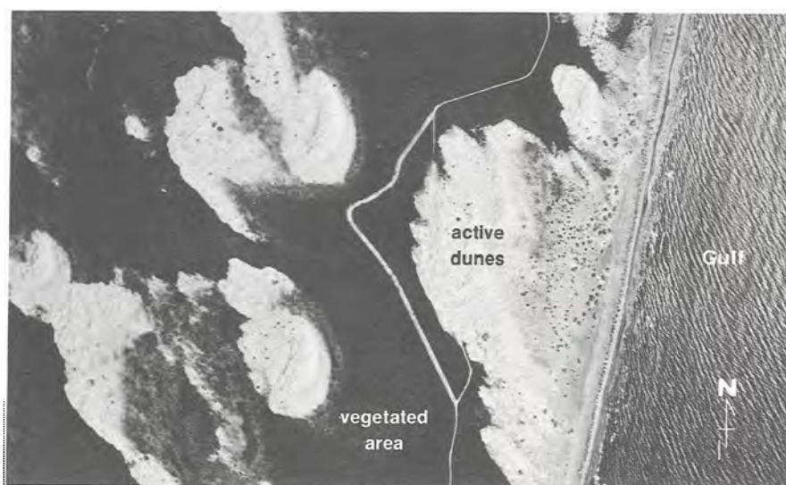
Figure 70. Road rerouted because of migrating dunes. Note the old road has been engulfed by active dunes that are migrating across the island. Gulf is to the right. Compare this figure (photograph taken in 1975) with figure 48 (photograph taken in 1974 before the new road was constructed).
