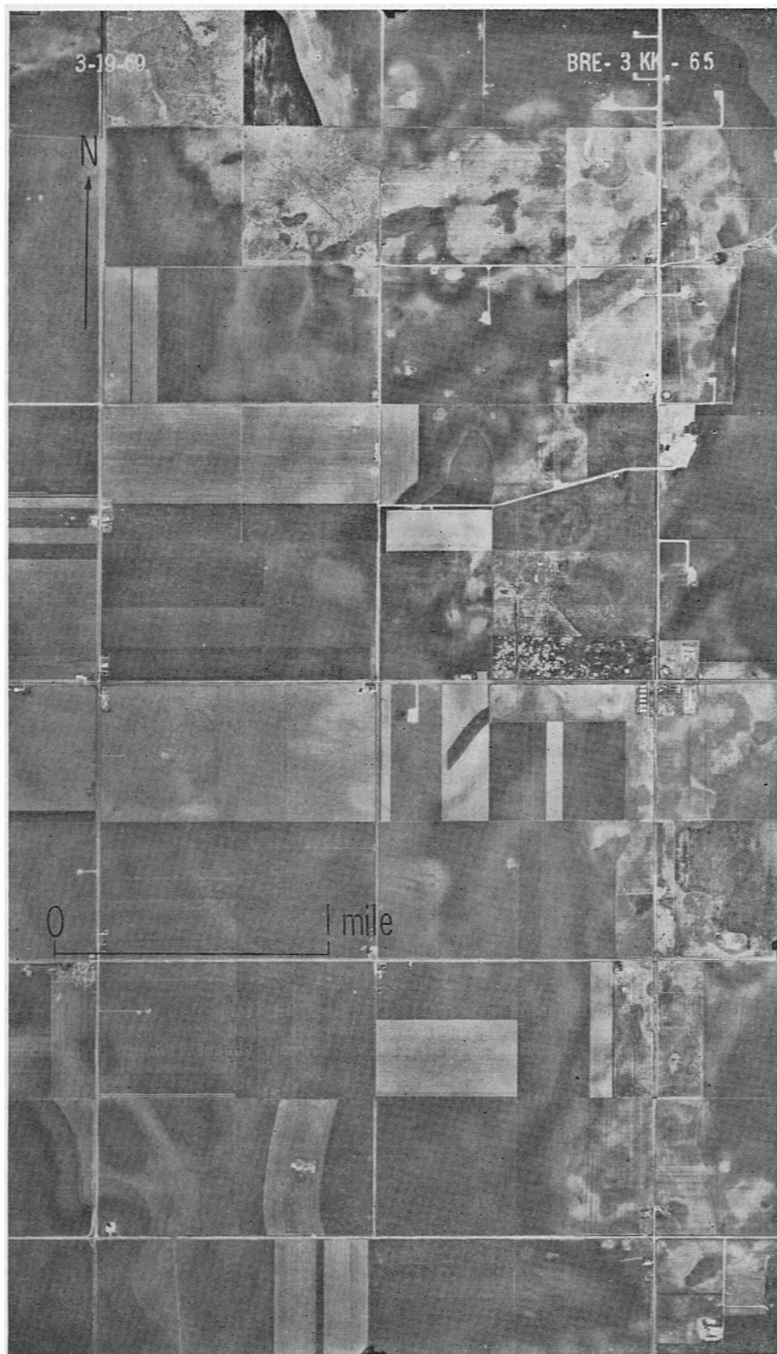
FIG. 6.—Air photo of part of distributary 2B (see Fig. 2). Light areas are underlain by loamy (sandy) soils. Dark circular and elliptical areas within lighter areas are shallow undrained depressions underlain by Banquette clay; dark area enclosing distributary, mainly Victoria clay. U.S. Dept. of Agriculture photo taken in 1969.
