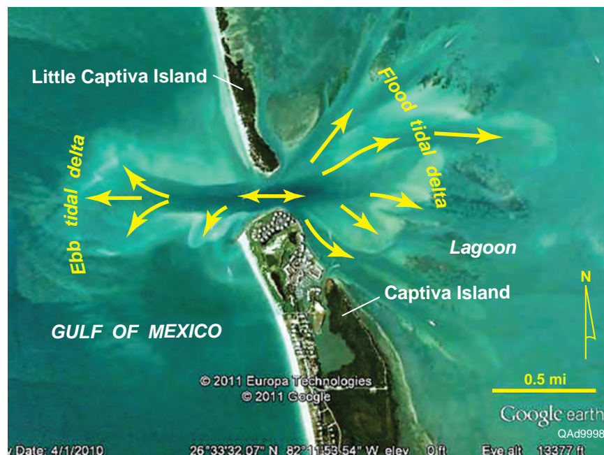
Figure 91. Tidal inlet between Captiva Island (south) and Little Captiva Island, Florida. Note the ebb-tidal delta (low tide) and flood-tidal delta (high tide). Arrows indicate tidal channels. Scale bar is 0.5 mile.
