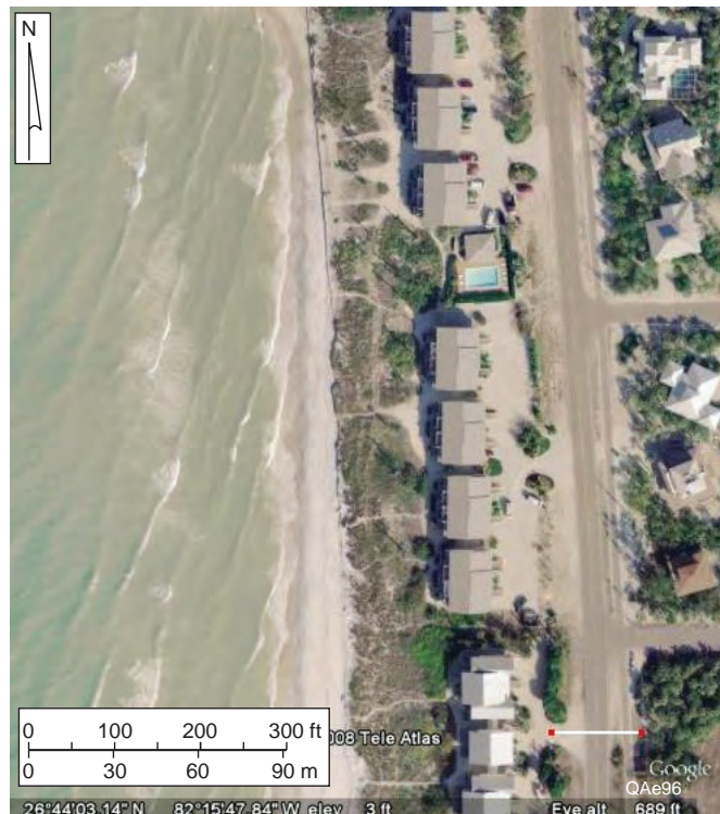
Figure 87. Waves strike the shore of Boca Grande, Florida, at an angle, producing a longshore current and longshore drift of sediment to the south (downward).
