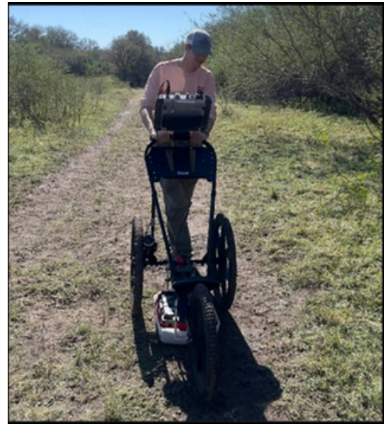
Jarrett Kernen (Mid-Coast TMN) surveys the Hackberry Trail Midden site with ground-penetrating radar in November 2025.
